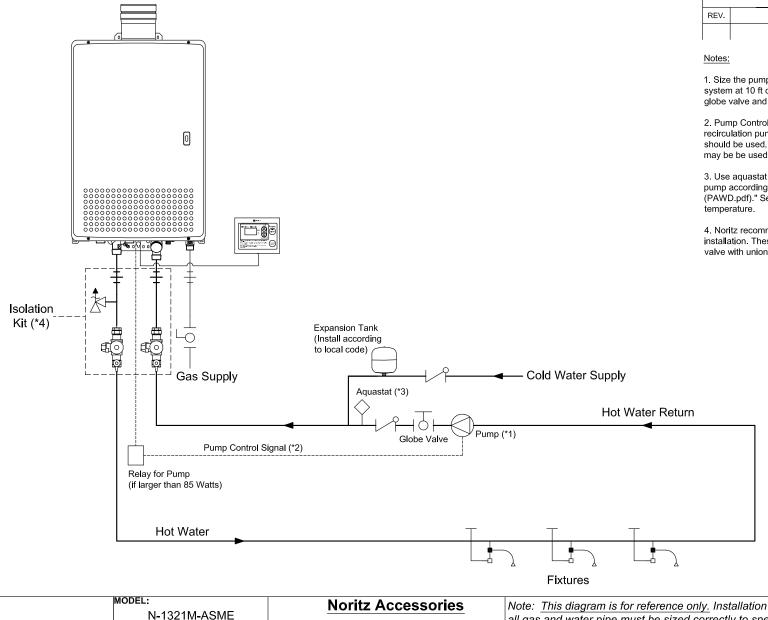
1. Size the pump to provide a maximum of 2 GPM through the system at 10 ft of head plus piping losses. Adjust the flow using a globe valve and verify the flow rate with the maintenance monitors.
